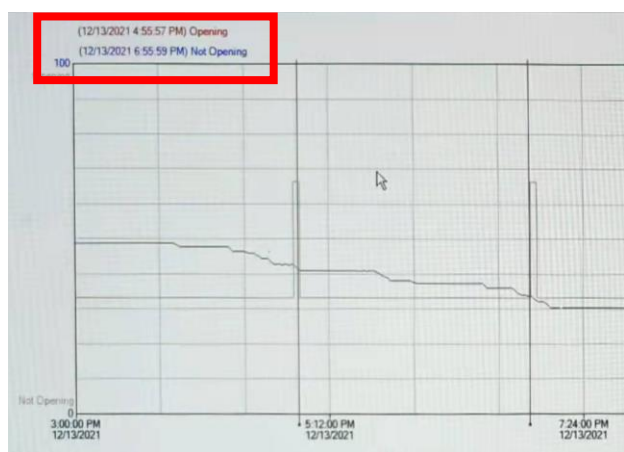
Automatic drainage per 2h when UOPs no PW request from UOPs in PW subloop1/2/3/4/5/6
